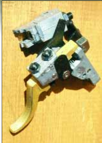
Above left, the trigger housing broke apart when the stock was removed. Right, a Timney Featherweight Deluxe trigger was a fine replacement.
