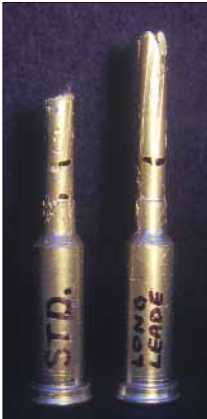
Left, chamber casts show the two different leads used in the test: factory SAAMI chamber and tapered lead (left) and factory chamber with modified straight lead to .250 inch (right). Below, the SAAMI chamber drawing.
