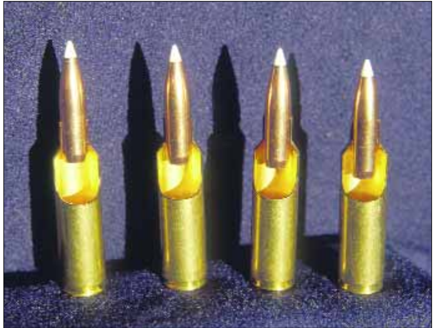
The .300 WSM cutaways show how far the bases of the bullets extend into the case at the four different OALs used in the test: (left to right) 3.000, 2.940, 2.880 and 2.820 inches.
