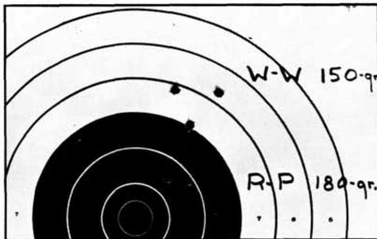
The 660 showed the classic tendency to place light bullets higher than heavy weights, as shown at the target at left, shot with the same centered hold on the bull. The 150-grain Silvertips hit about 2 3/8 inches higher than the 180-grain R-P Corelokts. The groups in the right photo were fired at 100 yards with the .308 barrel, and showed
