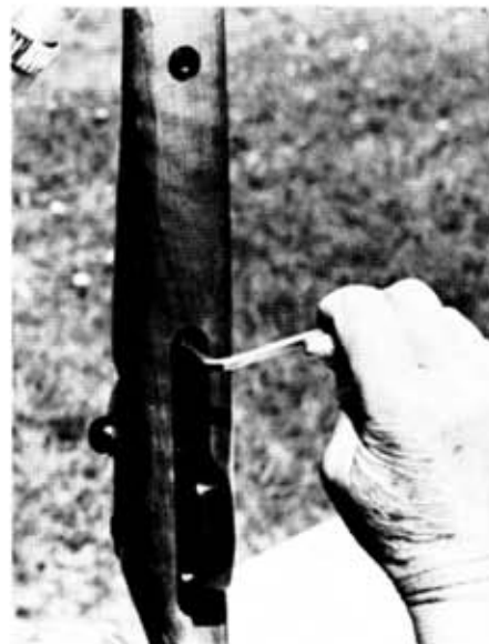
The Allen screws holding the barrel assembly allowed tightening with greater uniformity than would have been possible with screwdrivers, due to the leverage offered by the wrench.
