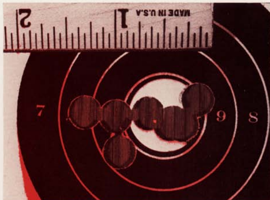
The 90-grain jacketed wadcutter, which is wider than it is long, gives surprising accuracy -- as this eight-shot 1 3/16-inch group fired at 100 yards shows. A light breeze blowing from 90 degrees apparently gave some horizontal dispersion.
