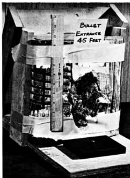
The destructive effect of the 90-grain jacketed wadcutter in the .357 Magnum rifle is evident in its effect upon a water-soaked Chicago phone directory. The entrance hole appears more like an exit hole, showing that the bullet blew up immediately upon contact with the book when traveling at about 2000 fps. Bullet fragments were found throughout the interior of the hole.
