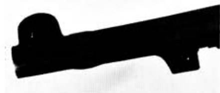
This S&W M1917 .45 revolver barrel is bulged just behind the front sight, probably caused by being fired with a bullet stuck in the bore. It is easily restored by cutting it off behind the bulge, truing up the muzzle, then fitting a new front sight.
