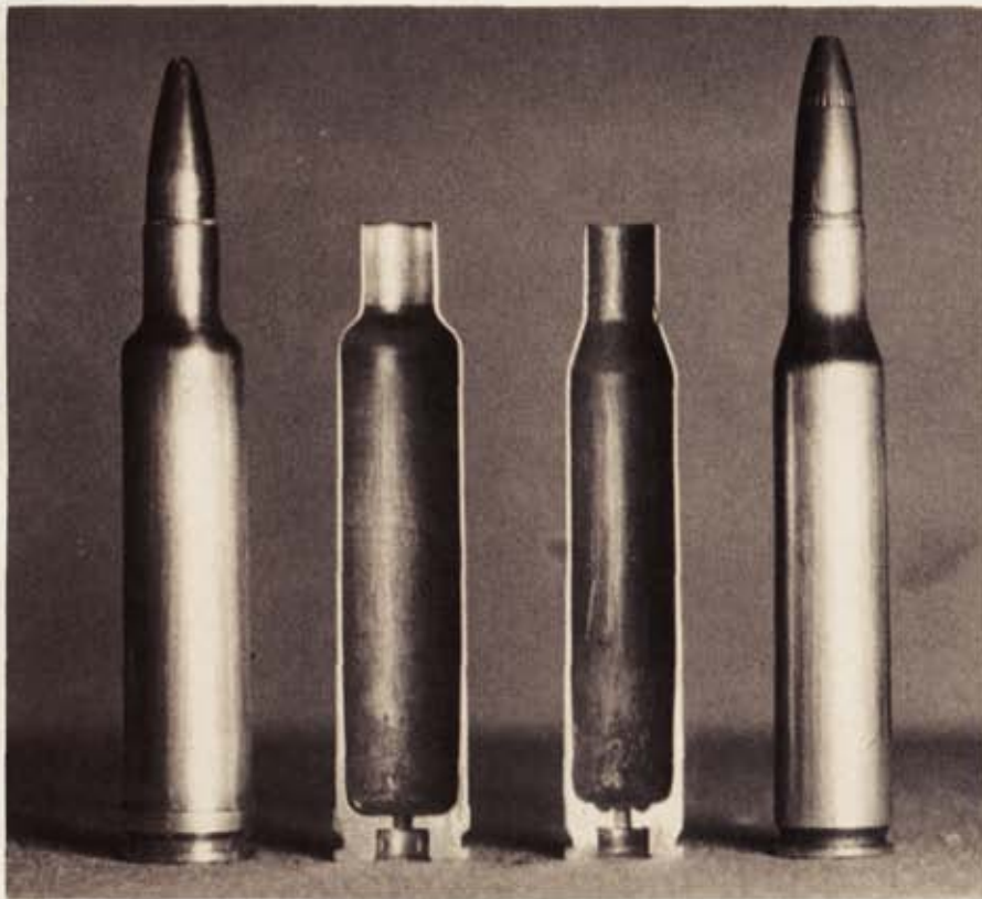
These sectioned .270 Weatherby Magnum and .270 Winchester cases clearly show why the .270 WM will take 77.5 grains of 4831 to the base of the neck, while the standard .270 WCF requires only 57 grains of 4831 to fill to the same level.
