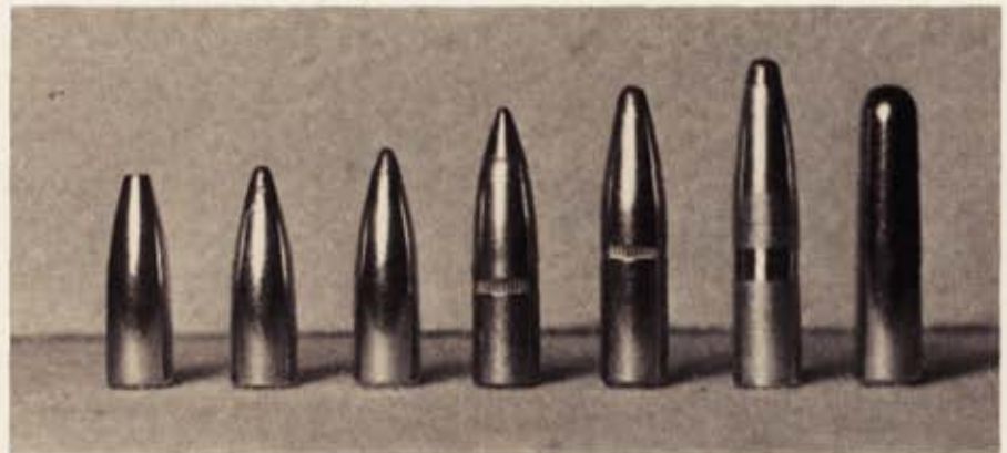
The wide range of bullets used in the tests include, from left, the 90-grain Sierra hollow point, 100-grain Speer Spitzer, 110-grain Sierra Spitzer, 130-grain Remington Bronze Point, 150-grain Hornady Spire Point, 160-grain Nosler semi-spitzer, and 170-grain Speer round nose.
