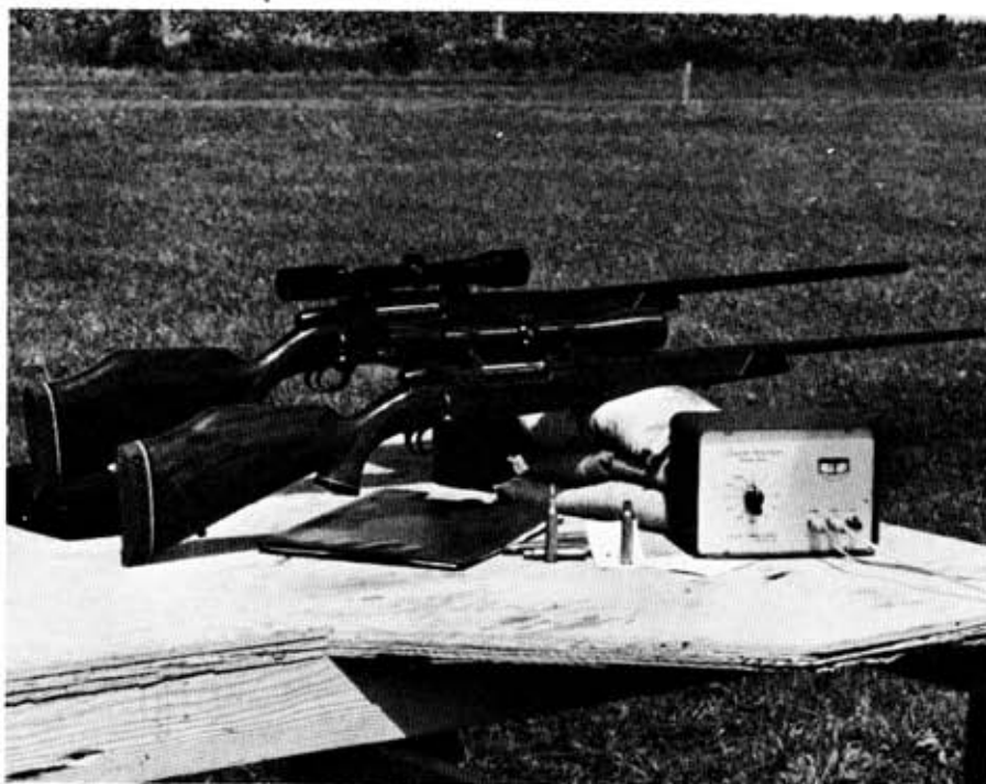
The author conducted extensive velocity and accuracy tests with this pair of .270 Weatherby Magnum rifles, finding that the 26-inch barrel model in the background often gave less additional velocity over the 24-inch tube than is generally supposed - with one load giving less velocity in the longer barrel. All velocities were checked on the accurate Model 10 Oehler chronograph shown.
